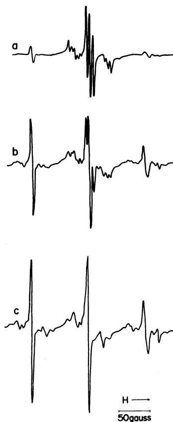
Fig. 5. The changes of ESR spectra of methyl isocyanate irradiated with \gamma -rays and exposed subsequently to visible light for 5 min (a), 30 min (b), and 90 min (c).
